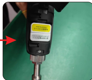
Insert the protective mirror holder into the chamber
