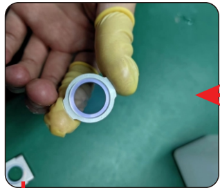
Insert the protective lens into the gland
