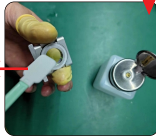
Wipe the front side of the protective lens with an alcohol-impregnated cotton swab or cloth.
