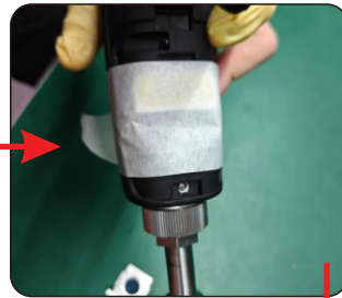
Tape the protective lens holder cavity
