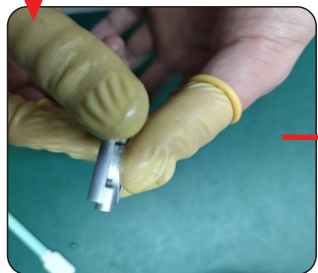
Align the gland with the protective lens drawer slot.
