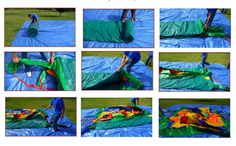
C. Unfold inflatable and locate zippers. Close all zippers and seal flap over zippers completely to make sure air is sealed.
