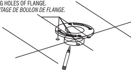
Put the flange on the drain hole, and fix it on the ground with four bolts. Then seal the flange with caulk.
