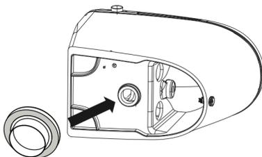
4. Install sealing flange into the drain outlet.
