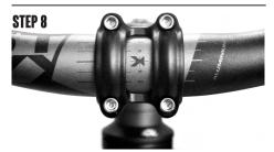
Center the handlebar and tighten the stem bolts in an "X" or cross pattern.
