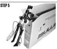
Lift the bike up and position it on the top of the BULLSBOX as shown above. Remove all packing material from the handlebars and fork.
