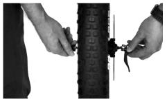
Make sure the brake's rotor is sitting on the left side of your bike and the quick release lever on the right side. Mount the front wheel onto your fork. Be careful not to damage the brake pads by applying too much force when mounting the front wheel.
