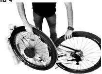
Remove the front wheel by detaching all packing cords and pulling it towards the front of the bicycle.
