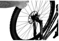
Insert the quick release through the fork and hub.
