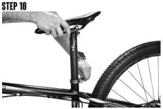
Now, slide the seatpost into the seat tube to the desired height. Make sure you DO NOT exceed the minimum insert line printed on the seatpost. Tighten it by either clamping down on the quick release lever or by using your BULLS hex to tighten it (this will depend on the model you have). Leave the plastic packaging on the saddle as you will need to flip your bike upside down and this will prevent any damage to your saddle.
