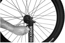
Make sure the brake's rotor is sitting on the left side of your bike and the quick release lever on the right side. Mount the front wheel onto your fork. Be careful not to damage the brake pads by applying too much force when mounting the front wheel.
