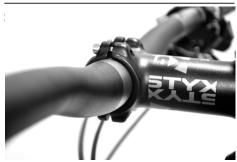
When tightening the bolts with the BULLS hex multitool or a torque wrench, tighten them alternately and equally to ensure that the faceplate is equally tight on every side. The gap between the faceplate and the stem should be equally wide on both the top and bottom.
