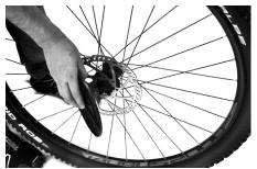
Pull the plastic protective caps off the axle from the front wheel.
