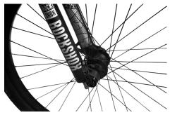
Tighten the quick release lever and make sure it points upwards (as shown in the picture above) so it does not open accidently by getting caught in branches or other objects.
