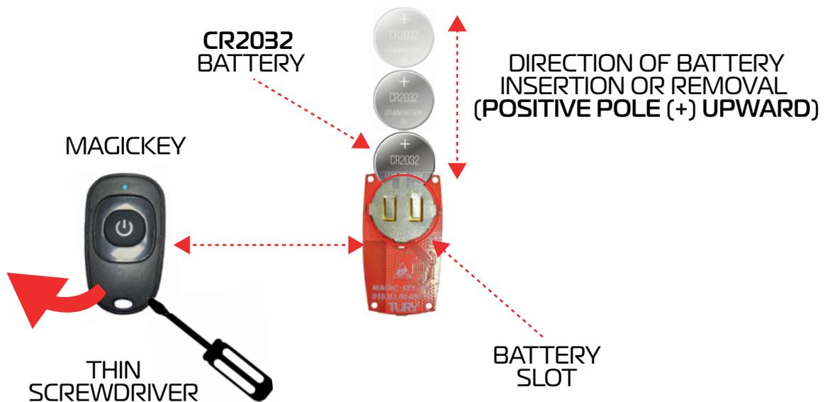
It is possible to monitor when the MagicKey's battery is low and time to be replaced, through the LED signaling of the MagicKey during its activation, where the led will flash twice for 10 seconds, or through the notification automatically generated on the home screen of the FAST MAX app.
