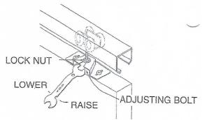
After final adjustment, tighten lock nut down to bracket as shown.
