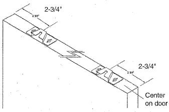
Screw brackets to top of door, 2-3/4" from edge of door, using 1-1/2" screws.
