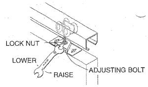
After final adjustment, tighten lock nut down to bracket as shown.
