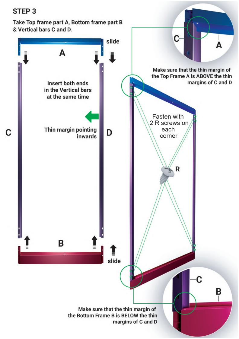
Insert the frame through the cabinet's walls slightly inclined. The side with rectangular holes must point inwards the cabinet.
