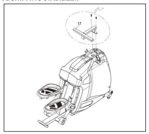
1. Use the Allen Wrench (119) to remove the two Bolts and discard the shipping stabilizer.
