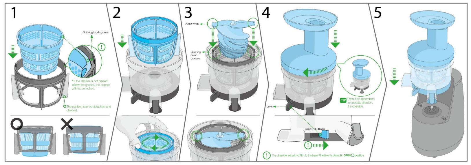
Assemble the strainer under the groove of spinning brush just like from the picture.
