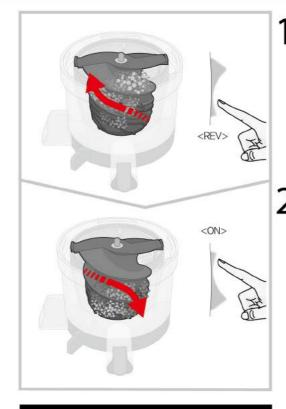
Press [Rev] button on the operating switch for 3~5 seconds and stop it. Repeat this 2~3times.
