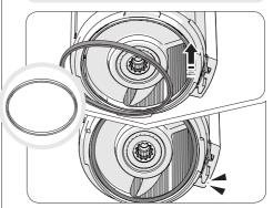
Assemble the packings as shown in the figure.
