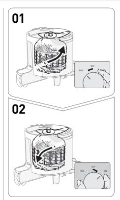
**01** For 2 to 3 times, repeat the process of maintaining the state in which the power dial is turned to the [REV] direction (counterclockwise) for 3 to 5 seconds and then releasing the dial. The reverse rotation is a function that returns and lifts the ingredients upward. It only works when the dial is being turned, and the screw rotation stops when the dial is released.
