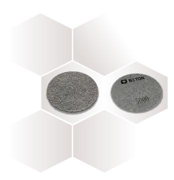
ULTRASHINE #5000 - Non Woven Pad is a superior quality rigid pad designed to optimize the polishing of natural stone surfaces. The unique material is developed to be used as a final grit to achieve brilliant gloss on dark material marble. To be used just with water to achieve high gloss without using any acidic powders or chemicals . Longer pad life makes the product highly economical to use.
