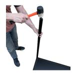
Please note: the connectors are designed to be tight and will usually require several firm hits with a rubber mallet to fully move into place. It's quite normal to shave off some plastic on the connectors as they are hammered into place.
