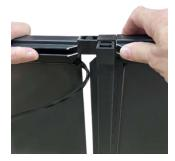
1. Line up the **Back Left** and **Back Right** side of the enclosure and then hammer the parts together using a rubber mallet. We recommend doing this by laying both pieces on a covered floor (to avoid scratching your enclosure) and placing one end up against a wall or solid object so that it's easier to hammer the parts together.
