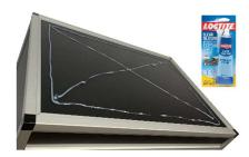
6. Rotate your enclosure so that it's on its top, then using the complimentary silicon, run it around all four sides and across the middle of the base, being careful to stay back at least 1 inch from the edges as shown. Now guide the last panel into position to fully reinforce the base of your new enclosure.
