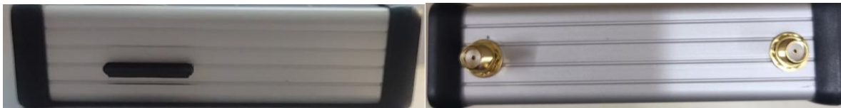
Option 2 – Remote installation option with Dual Antennas for GPS and ADS-b in
