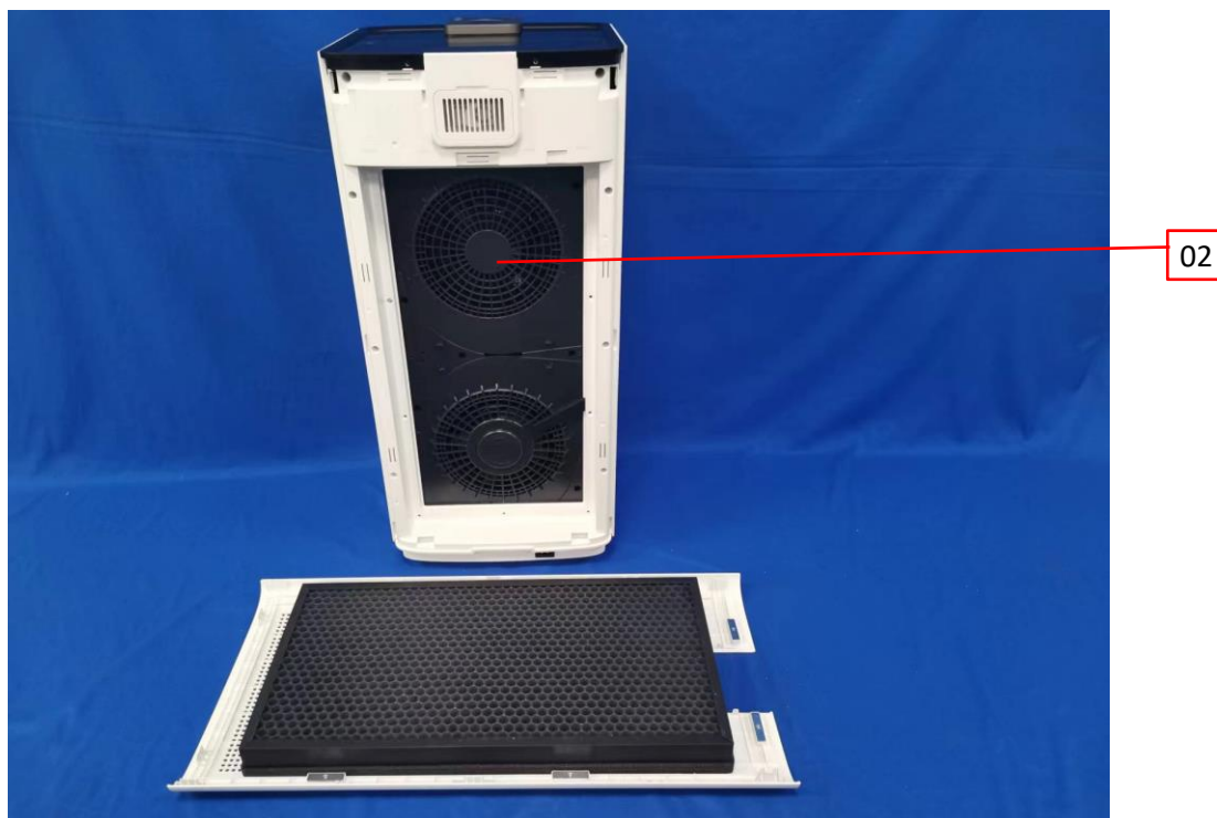
Photo 5 - Internal view with filter removed
