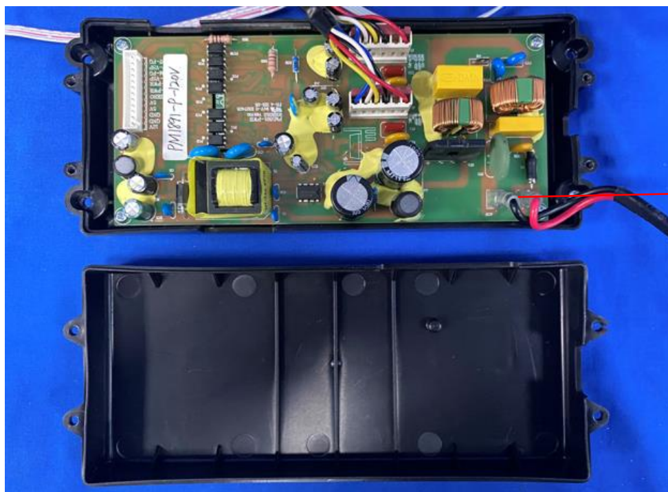
Photo 18 - Internal view of PCB box
