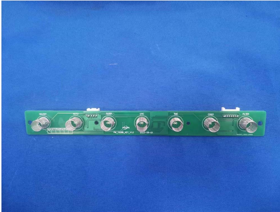
Photo 19 - PCB of keyboard view
