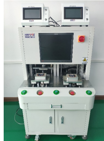
Air tightness test
