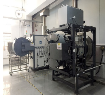
EP catalytic debinding equipment
