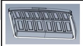
**Apply included** gasket to the outside edge of the RotoKap base as shown. In white
