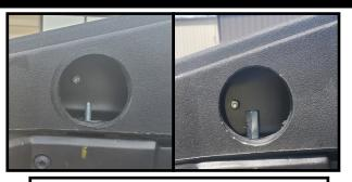
Re-attach the previously removed Washer and Coupling Nut to each of the 4 "Plug Inserts" and tighten with 3/8" wrench.
