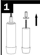
**Remove: Washers and Coupling** nuts from all 4 "Plug Inserts" and set aside. [Plugs will have a different shape for Defender, hardware and assembly are the same
