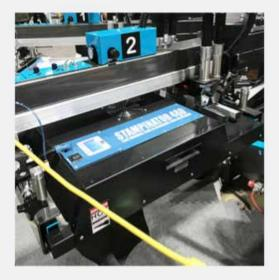
Bring the print head assembly down and lock the unit in place. Be sure to move the print carage to the rear of the unit, as well as moving the print head PROX. Lock down the air cylinders and tighten the manual clamp downs for added locking pressure.
