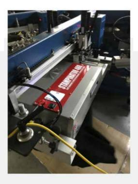
Bring the print head assembly down and lock the unit in place. Be sure to move the print carage to the rear of the unit, as well as moving the print head PROX. Lock down the air cylinders and tighten the manual clamp downs for added locking pressure.
