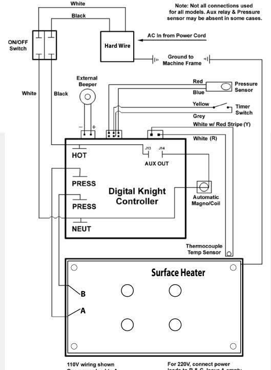
One power lead to A Other power lead to B & C joined leads to B & C, leave A empty
