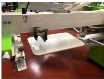
Bring the print head assembly down and lock the unit in place. Be sure to move the print carage to the rear of the unit, as well as moving the print head PROX. Lock down the air cylinders and tighten the manual clamp downs for added locking pressure.
