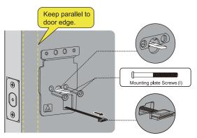
B Secure the mounting plate with the supplied screws. Do not overtighten screws.
