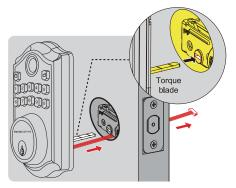
A With the latch fully retracted (in the unlocked position), route the cable below the latch, and insert the torque blade through the slot in the
