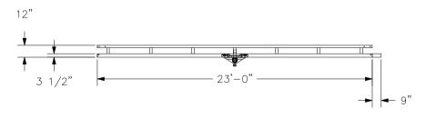
⊗ = HANGER POINT DO NOT SCALE FROM DRAWING. DIMENSIONS ARE STEEL TO STEEL AND MAY VARY. HANGER POSITION TOLERANCE = ±3 1/2"
