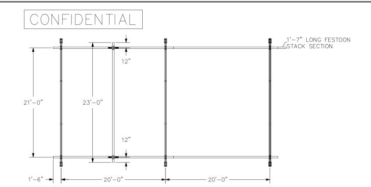
SUPPORT ASSEMBLIES ARE DESIGNED TO AISC SPECIFICATIONS. IF NO MOVEMENT OF SUPPORT ASSEMBLIES IS REQUIRED, THEN BRACING TO BUILDING STEEL IS RECOMMENDED (NOT INCLUDED).
