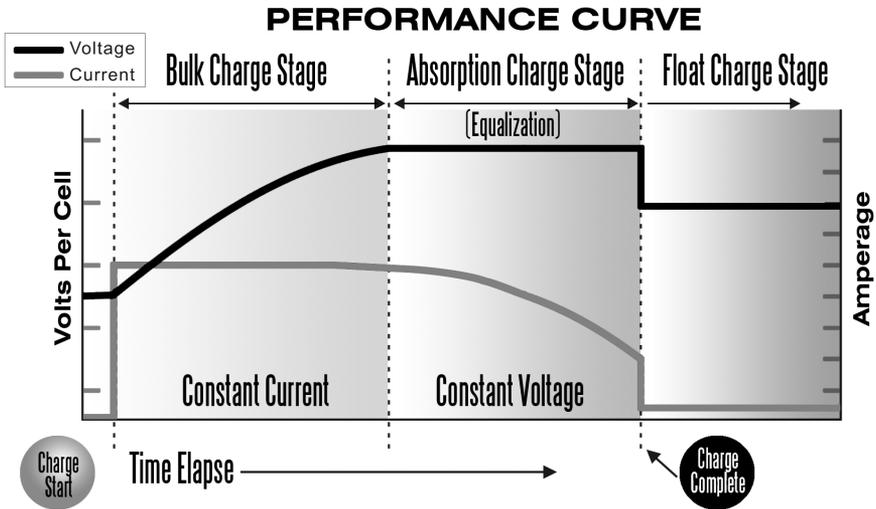
Figure B-1 Three-stage charging profile
