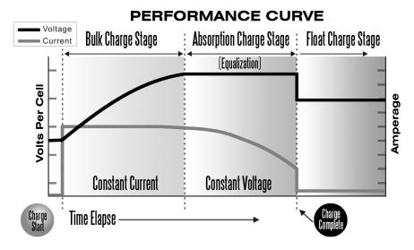
Figure B-1 Three-stage charging profile
