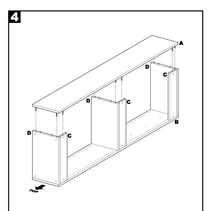
**4.1** Install Left Side Panel (A) onto assembled Set Shelves (D) and Rear Hanging Cleats (C). BE SURE Wood Dowels in Shelves and Cleats engage drilled holes in Side Panel, and Side Panel is pressed flush against Set Shelves and Cleats.
