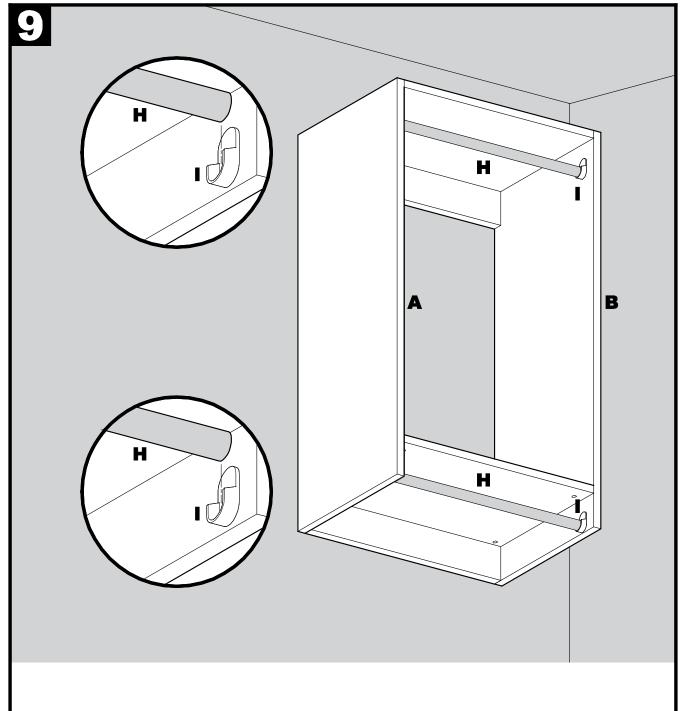
NOTE: Use care when installing Hanging Rods (H) to avoid scratching finish inside unit.
