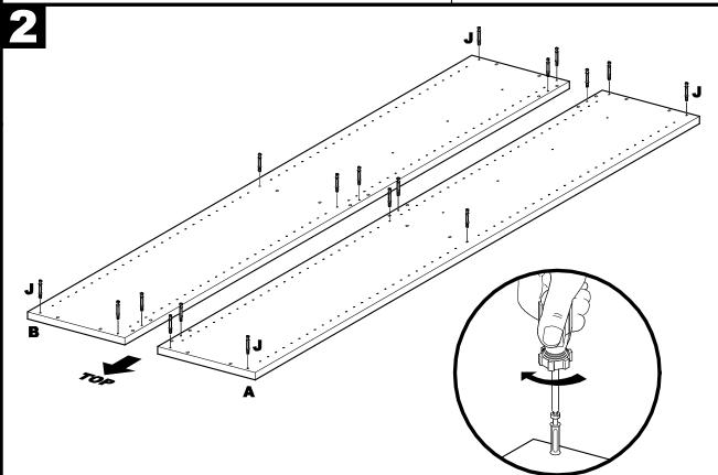
2.1 Install one Cam Post (J) into each of the nine holes on Left Side Panel (A) and Right Side Panel (B). Tighten until Cam Posts are seated against Side Panels.
