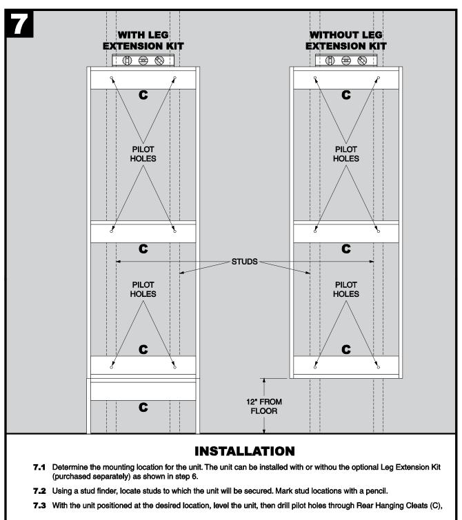
**NOTE:** For units under 25-1/2 inches wide, it is likely that only one stud will pass through the unit. In these cases, use two screws through each Rear Hanging Cleat.
