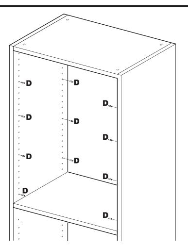
**4.1** For each Shoe Shelf, insert two front Duplo Pins (D) into pin holes inside of Tower at the desired height, then install rear Duplo Pins (D) two holes higher than the associated front pins.
