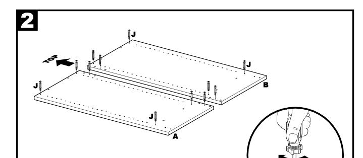
2.1 Install one Cam Post (J) into each of the six holes on Left Side Panel (A) and Right Side Panel (B). Tighten until Cam Posts are seated against Side Panels.
