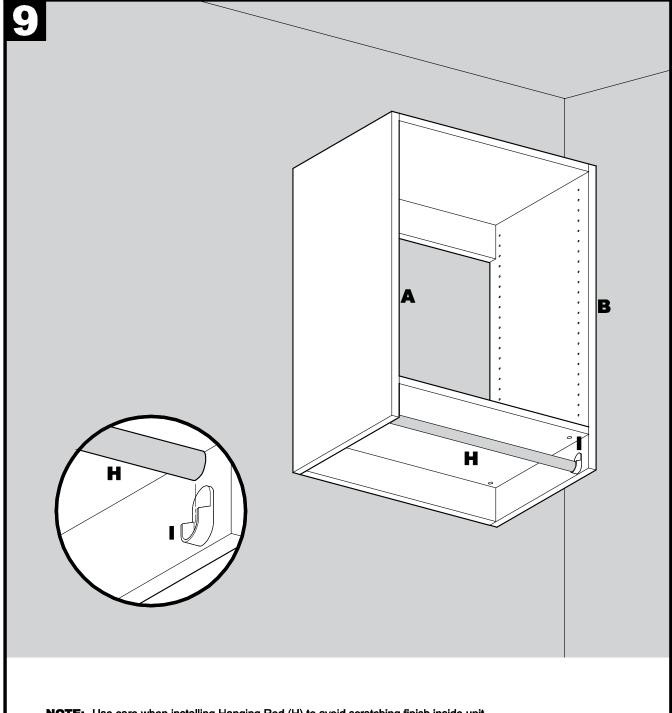
NOTE: Use care when installing Hanging Rod (H) to avoid scratching finish inside unit.
