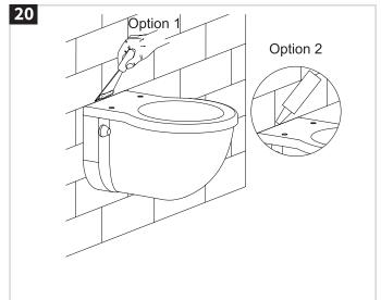
Once pan is installed, check for function and leaks. Once complete seal the joint between the pan and wall as appropriate.
