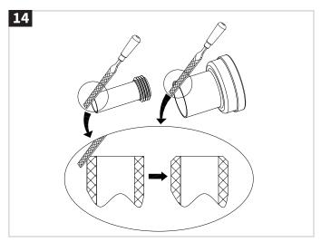
Chamfer and deburr pipe ends as appropriate.
