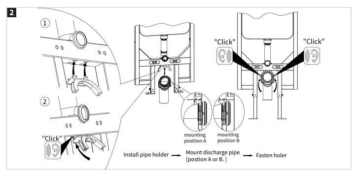
Connect the waste outlet pipe to the frame as shown.
