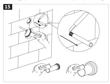
Cut the protection sleeve outside of the wall with a knife.
