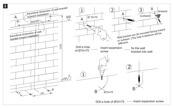
Drill the holes and insert the expansion bolt. Note: Above are theoretical dimensions of the frame, please follow the practical location of frame.
