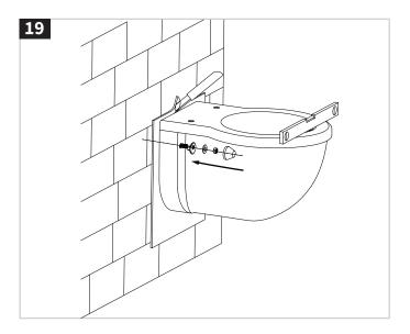
Once flush and waste pipes are properly seated secure the pan to the wall/frame with fixings supplied.
