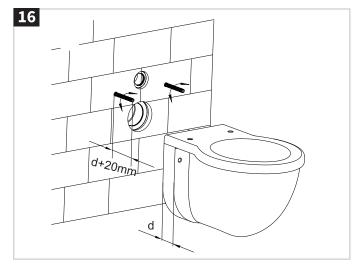
Adjust length of connecting bolt to be d+20mm
