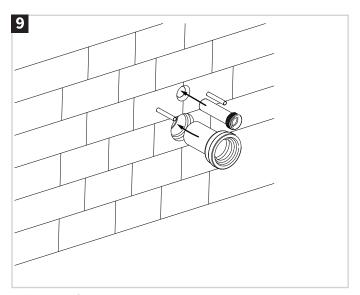
Fully insert flush and waste pipes.
