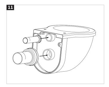
Connect flush and waste pipes to pan.
