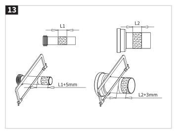
As per drawing, L1 is distance between the two lines on straight tube. L2 is the distance between the two lines on conecting pipe. Cut the flush and waste pipes per drawing
