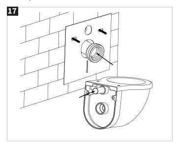
Insert flush pipe connector in pan and waste pipe connector to frame.
