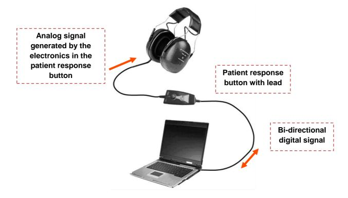
The DSP (Digital Signal Processor) located in the patient response button ensures communication with both the computer and the sound generation.
