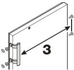
4. Transfer pin on hinge bracket to the opposite side.
