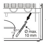
Drill marked section on the back of the appliance.
