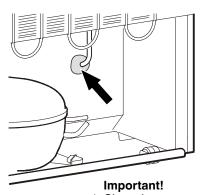
4. Close the sensor cable opening at the back of the appliance with the sealant provided.
