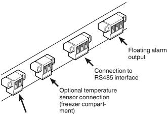
Optional temperature sensor connection (refrigerator compartment)
