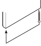
15. Suspend the freezer door on the hinge pin and close.
