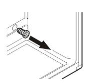
Pull out strain relief device.
