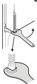
10. Reinstall the middle hinge bracket on
