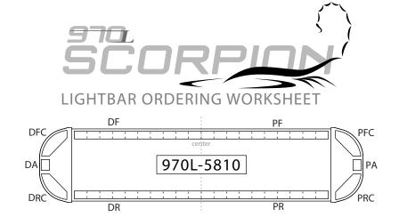
The front of the 970L-5810 is limited to 10 lamp positions not including blanks. This means that for bar that is full with no blanks could accommodate 6 full lamps and 4 - 1/2 lamps. Blanks may be 1/2 or full size or any combination of both. LED warning lights are also available for 1/2 lamp positions. Full and 1/2 LED warning lamps are available in red, blue, amber and white LEDs and lens colors.
