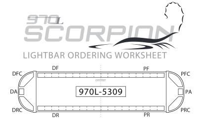
The front of the 970L-5309 is limited to 10 lamp positions not including blanks. This means that for bar that is full with no blanks could accommodate 6 full lamps and 4 - 1/2 lamps. Blanks may be 1/2 or full size or any combination of both. LED warning lights are also available for 1/2 lamp positions. Full and 1/2 LED warning lamps are available in red, blue, amber and white LEDs and lens colors. All Dual Color lamps come with a clear lens.
