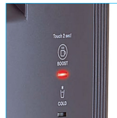
Hot water booster button to raise the temperature from 90°C to 95°C (Limited quantity)
