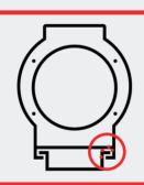
\*BEFORE REMOVING KIEF TRAY, BRUSH EXCESS KIEF OFF THE INSIDE LEDGES WHICH HOLD TRAY IN THE MACHINE \*
