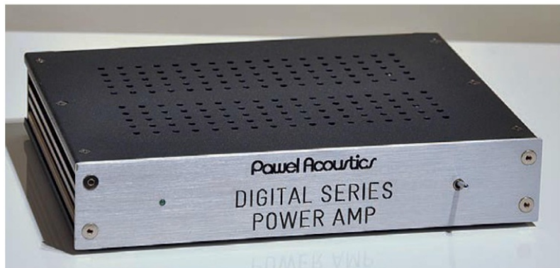
Here is a 6-kilo, 250-watt digital power amplifier from 1984.
