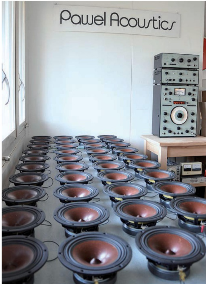
A picture from today: these drivers are 'burned in' around the clock in the factory.
