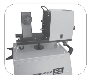
Carefully place the wire-feed unit onto the support column.
