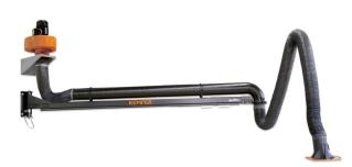
Length: 7 m, Ø 150 mm~ (without filter)~ Fan 2,000 m³/h~ 1.1 kW~ 3x400 V Extraction capacity: 1,000 m³/h Length of extraction arm: 4 m Length of boom: 3 m (type 79 007 201)
