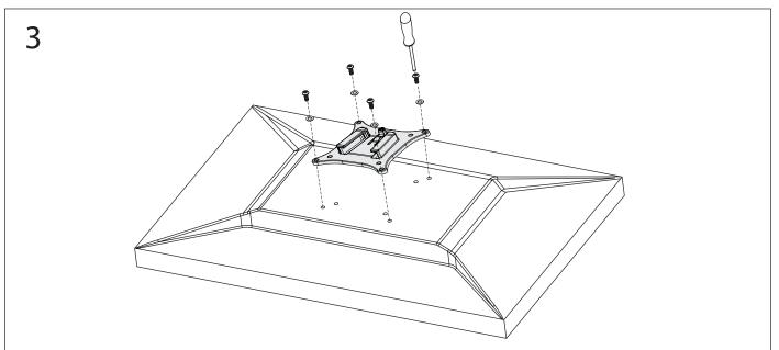
Lay your monitor face down and align the VESA plate with the arrow pointing towards the top of your screen and fix using the screws provided and a phillips head screwdriver.
