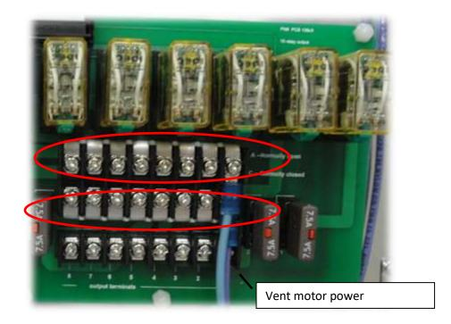
Bus can be reduced or removed to allow fans, heaters, or lights to be connected instead of vent motors. To shorten them, remove the connector completely then use pliers to snip it to length.
