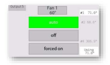
The overrides allow you to force an output. In Auto, it will operate automatically. Selecting Off or Forced allows you to avoid the control system. The app's temperature is shown. All contributing probes are highlighted.
