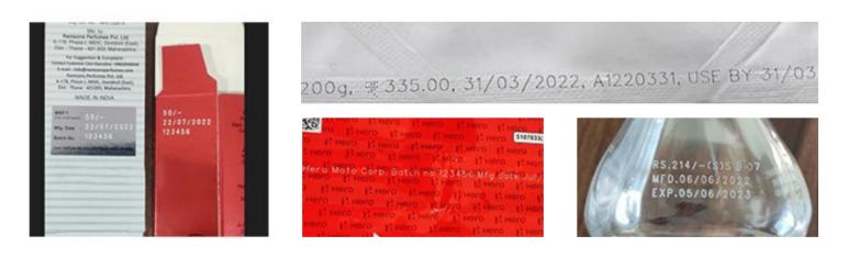
One of the biggest appeals of laser coding systems is their ability to mark substrates moving at high speeds up to 2,000 characters per second. With these speed capabilities, businesses involved in large-scale packaging and manufacturing can make sure that all of their products are marked with the necessary text and codes to comply with traceability standards and state/federal regulations
