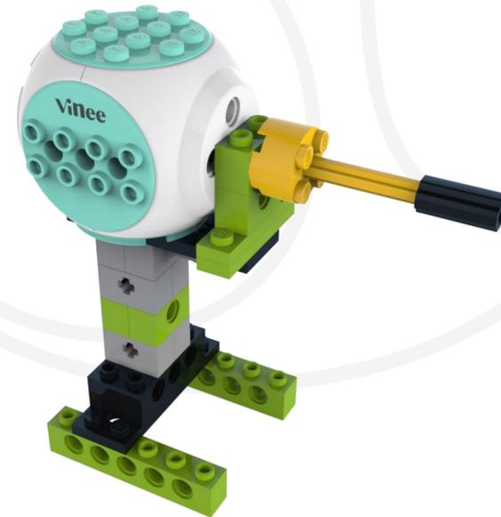
**Description:** Learn how an electric motor changes electrical energy into mechanical movement to power the drill. Observe the rotational motion of the Axle and experiment with motor direction.
