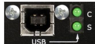
Note: Microsoft Windows® only supports USB Audio Class 1, so that in Windows operating systems the sampling rates of 176.4 and 192 kHz are available with 16 bit resolution only.
