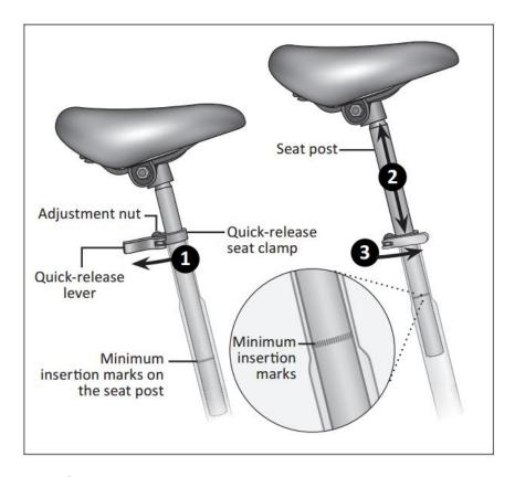
A loose seat clamp or seat adjustment bolt can cause loss of control, bike/property damage, serious injury, or death. Regularly check to make sure that the seat adjustment bolt is properly tightened and the clamp is secure on the seat rails.
