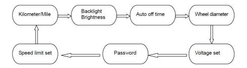
*Kilometer/Mile* – Symbol on display S7. Press Up/Down to rotate between mph and km/h.
