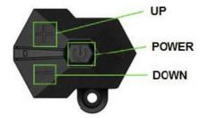
Press the power button (left button) on the four button selector located near the left grip on the handlebars to turn the meter on. You can adjust the pedal assist power level to have more power by hitting the [+] button (top button) and can move to a lower level power by hitting the [-] button (button button).
