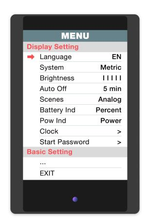
**System** - Press **Up/Down** to switch between Metric / Imperial.
