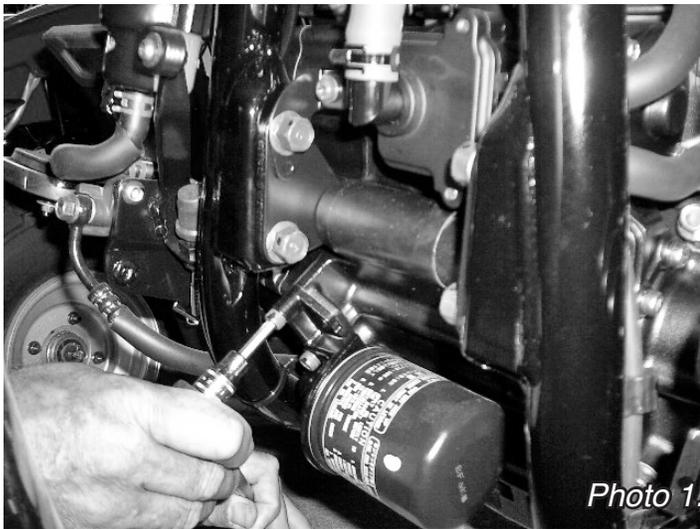
**NOTE:** The oil filter may be left in place during the installation (Photo 2) if desired. If removed, however, the oil must be drained from the oil filter and all mounting surfaces must be cleaned of oil and dirt.
