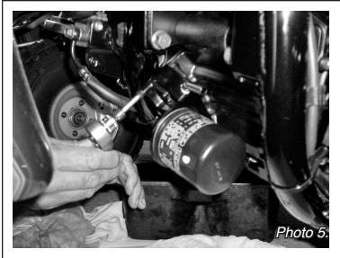
12. The 4800 Jagg oil filter adapter is now installed (Photo 6).
