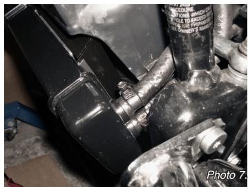
**TIP**: Install 7/8" black hose clamps loosely onto hoses before installing hoses onto oil cooler nipples. A touch of oil on oil cooler nipples allows the hoses to push on easily.
