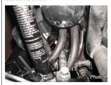
40. Install oil filter onto the threaded stem of the oil filter adapter. Tighten per factory/service manual recommendations.
