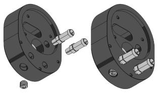
Wrench tighten the plug to 2-3 turns-from-finger-tight (T.F.F.T.).
