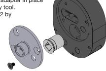
hex key tool. Then, remove the faceplate from the adapter and remove the LOCNUT from within.
