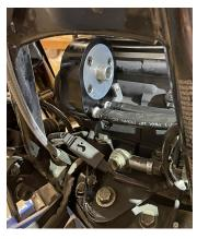
ensure hose clamps do not interfere with oil filter installation.
